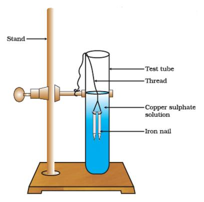
(i) Describe the setup of the experiment where iron nails are dipped in copper sulfate solution.
